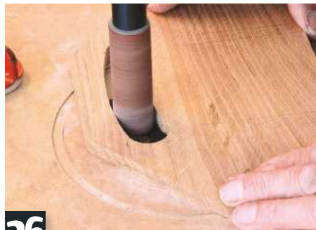
26 Clean up cutout with 25mm sanding drum or rasp and file. Smooth edges with abrasives
